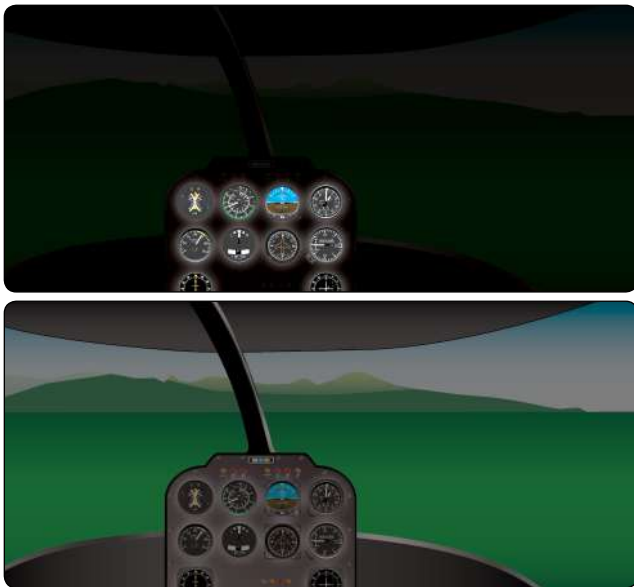
Figure 12-1. Effects of dimming cockpit lighting during night flight to better see surrounding terrain.
