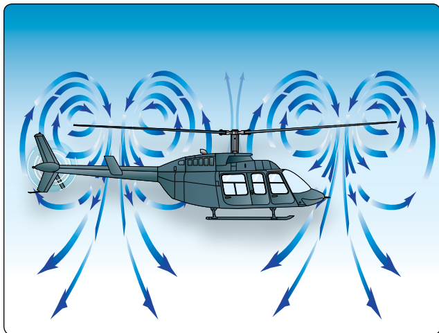
Figure 11-3. Vortex ring state.
