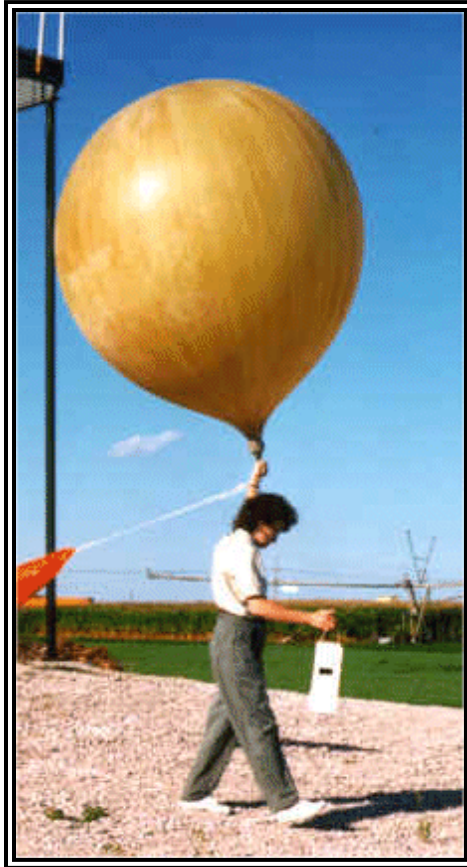
Figure 5-8. Weather Balloon and Radiosonde
