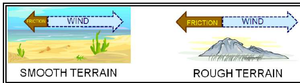
Figure 7-6. Friction Force Magnitude Variations with Terrain Roughness
