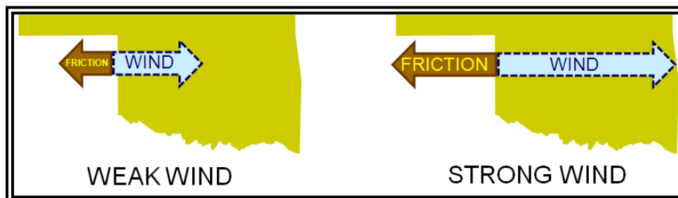
Figure 7-7. Friction Force Magnitude Variations with Wind Speed
