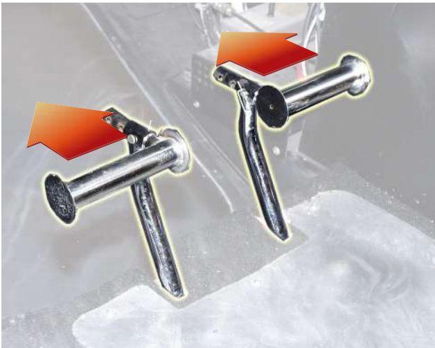
Figure 3-5. Antitorque pedals compensate for changes in torque and control heading in a hover.
