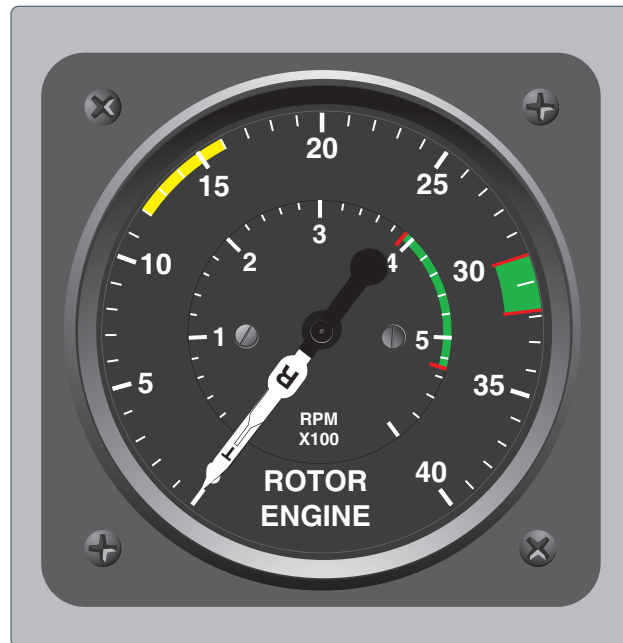
Figure 5-3. Markings on a typical dual-needle tachometer in a reciprocating-engine helicopter. The outer band shows the limits of the superimposed needles when the engine is turning the rotor. The inner band indicates the power-off limits.
