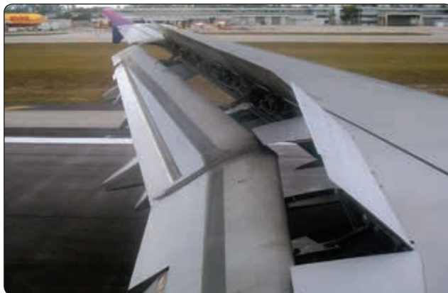
Figure 6-19. Spoilers reduce lift and increase drag during descent and landing.
