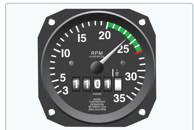
Figure 7-8. Engine rpm is indicated on the tachometer.
