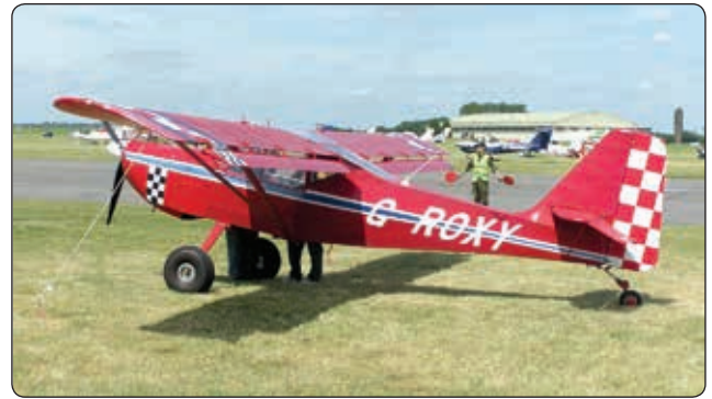
Figure 6-9. Flaperons on a Skystar Kitfox MK 7.
