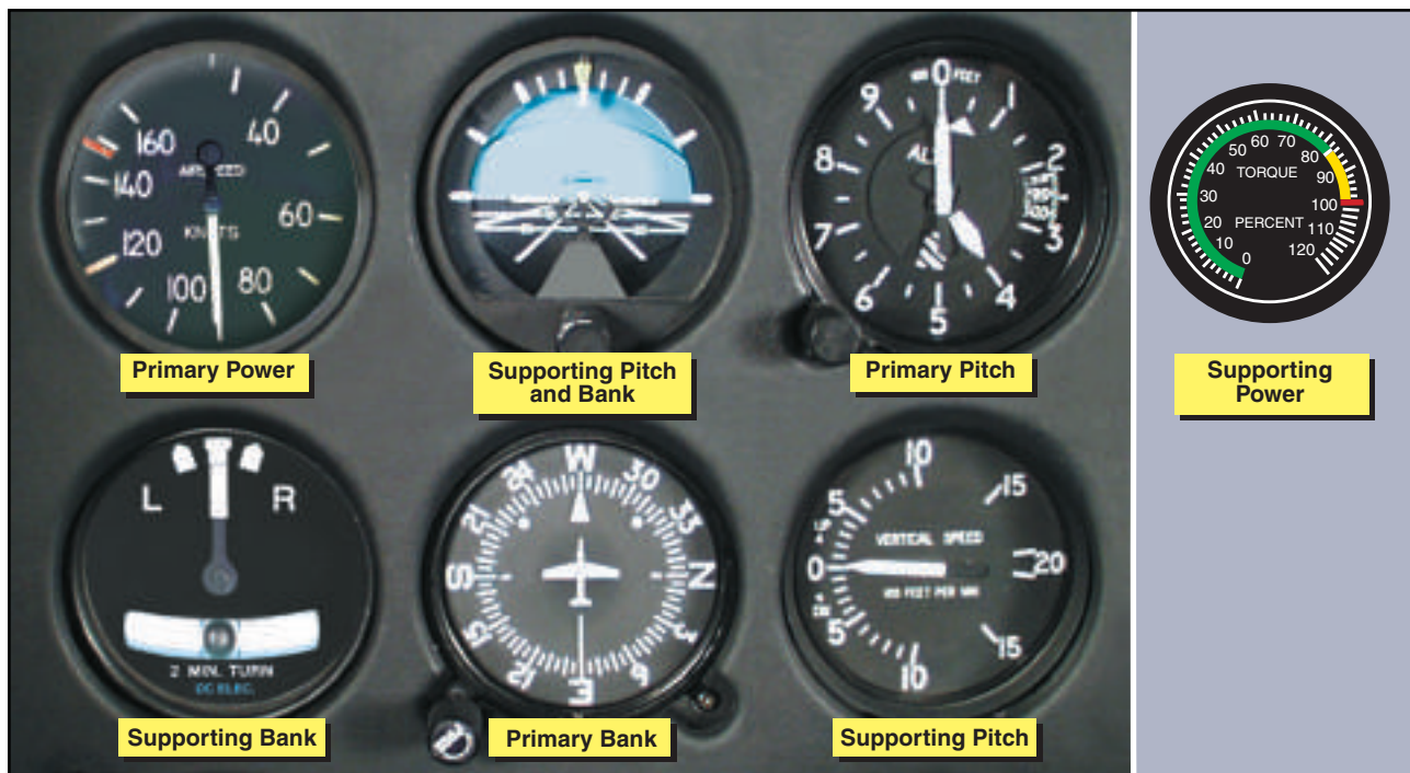
Figure 12-15. Flight instrument indications in straight-and-level flight at normal cruise speed.
