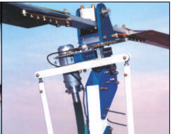
Figure 17-1. A common method of transferring cyclic control inputs to the rotor head is through the use of push-pull tubes, located outboard of the rotor mast pictured on the right.
