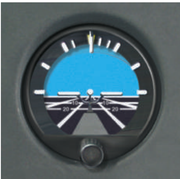
Figure 12-12. The initial pitch correction at normal cruise is one bar width.
