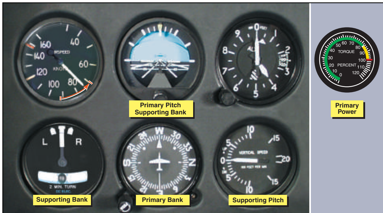
Figure 12-17. Flight instrument indications during climb entry for a constant airspeed climb.
