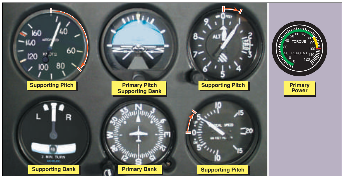
Figure 12-22. Flight instrument indications during an instrument takeoff.
