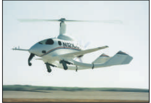
Figure 15-3. The CarterCopter uses wings to enhance performance.
