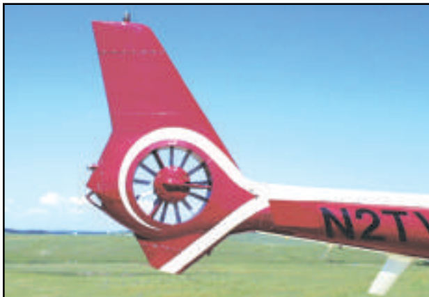
Figure 1-4. Compared to an unprotected tail rotor, the fenestron antitorque system provides an improved margin of safety during ground operations.
