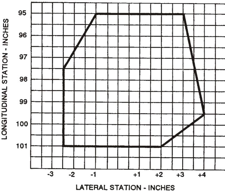
Figure 2-2. Center-of-Gravity Envelope
