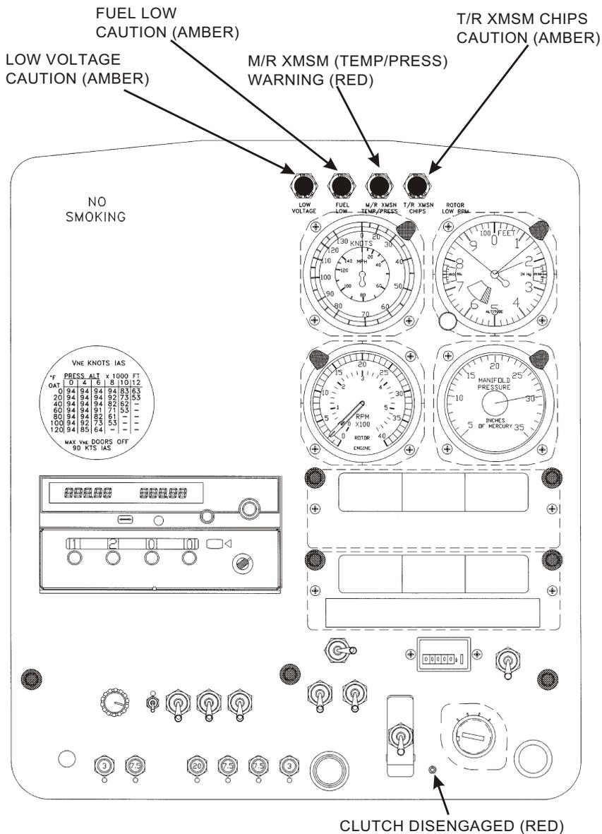
Figure 3-1A. Instrument Panel - Warning/Caution Lights (Helicopters with fuel injected engine - HIO-360-G1A)
