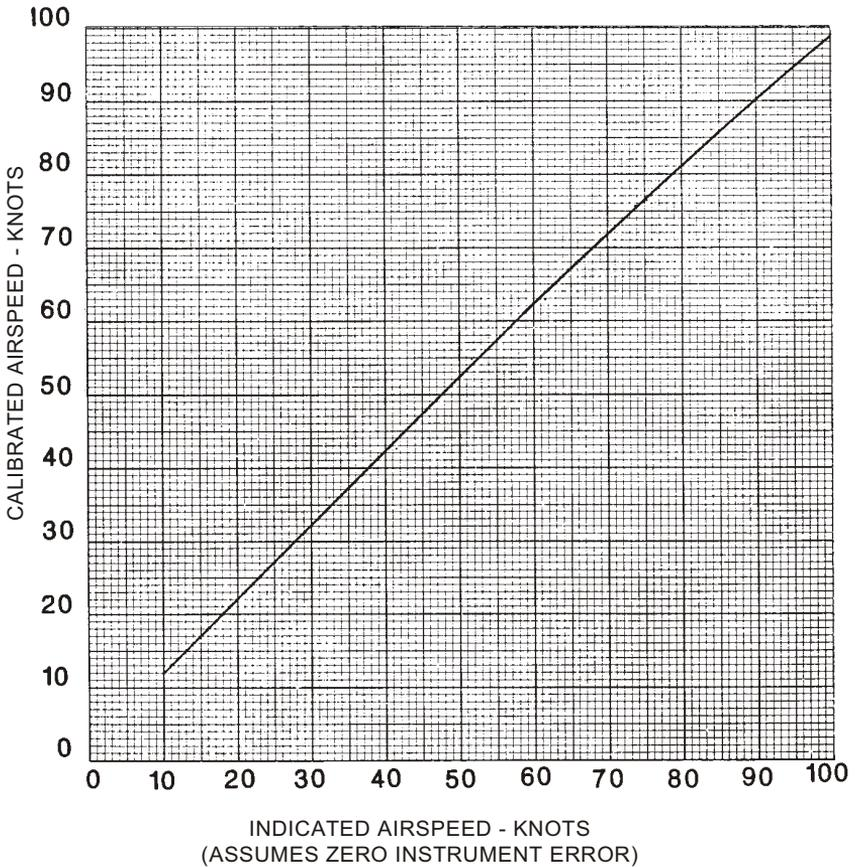
Figure 5-1A. Airspeed Calibration Curve - Heated Pitot Tube
