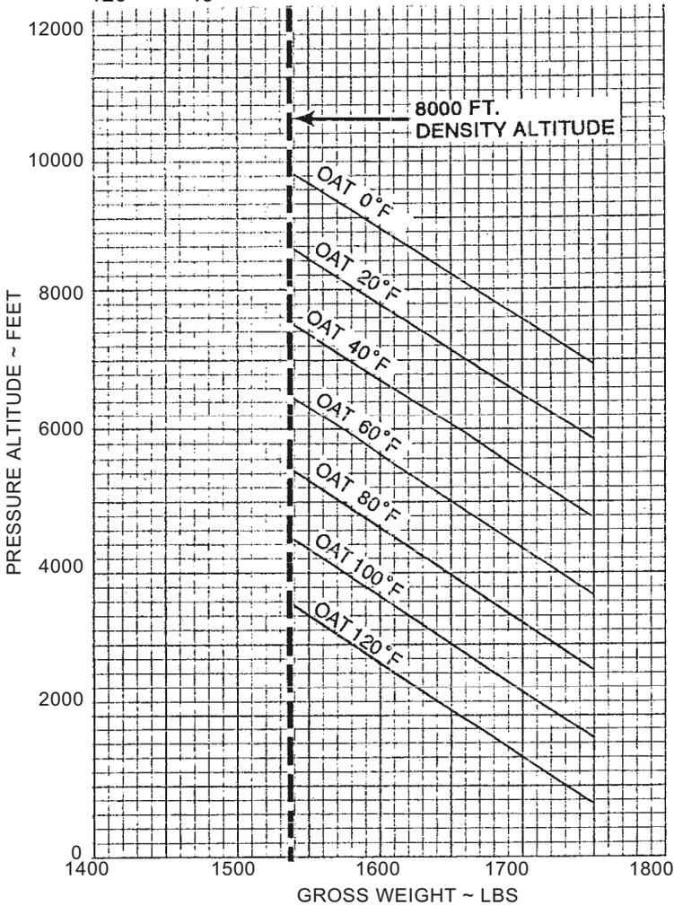
Figure 5-4A. In Ground Effect Hover Ceiling Versus Gross Weight (Helicopters with fuel injected engine - HIO-360-G1A)
