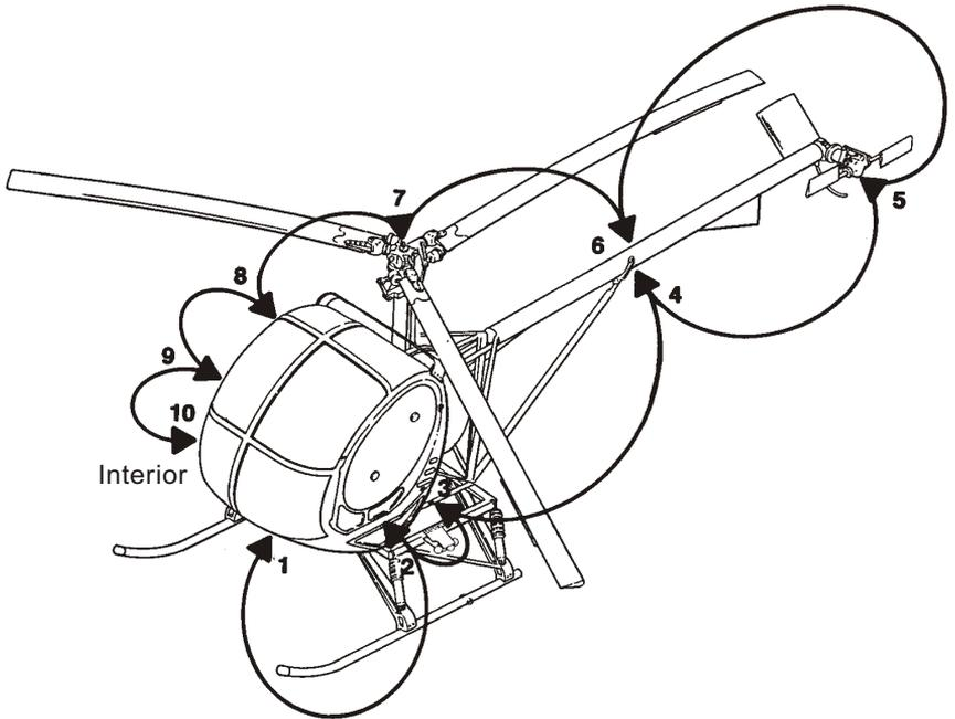
Figure 4-1. Pilot's Preflight Guide
