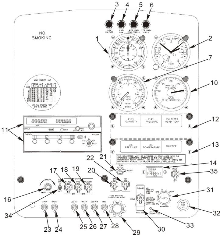
Figure 4-2B. Typical Instrument Panel Configuration (Helicopters with fuel injected engine - HIO-360-G1A)
