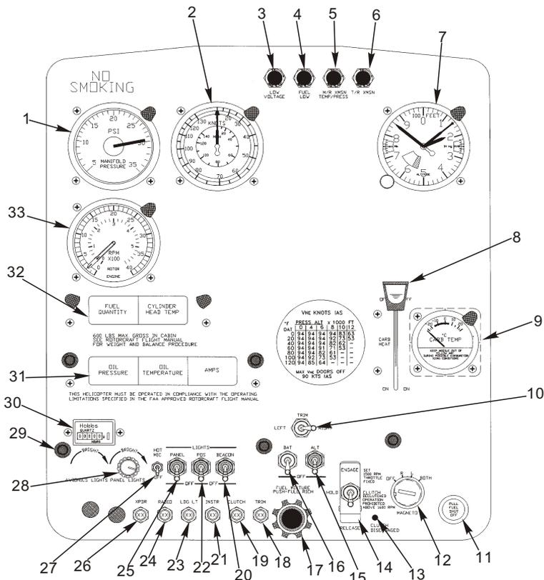
Figure 4-2A. Alternate Instrument Panel Configuration
