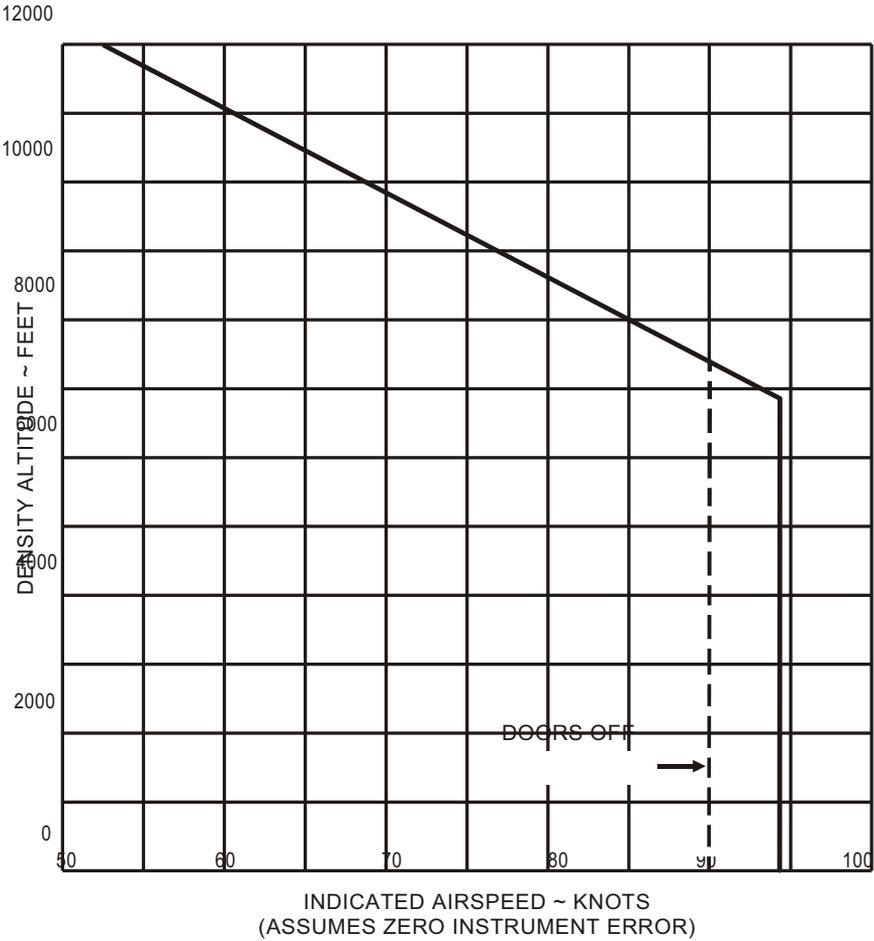
Figure 2-1. Variation of  $V_{NE}$  with Altitude at 1750 lbs. Gross Weight
