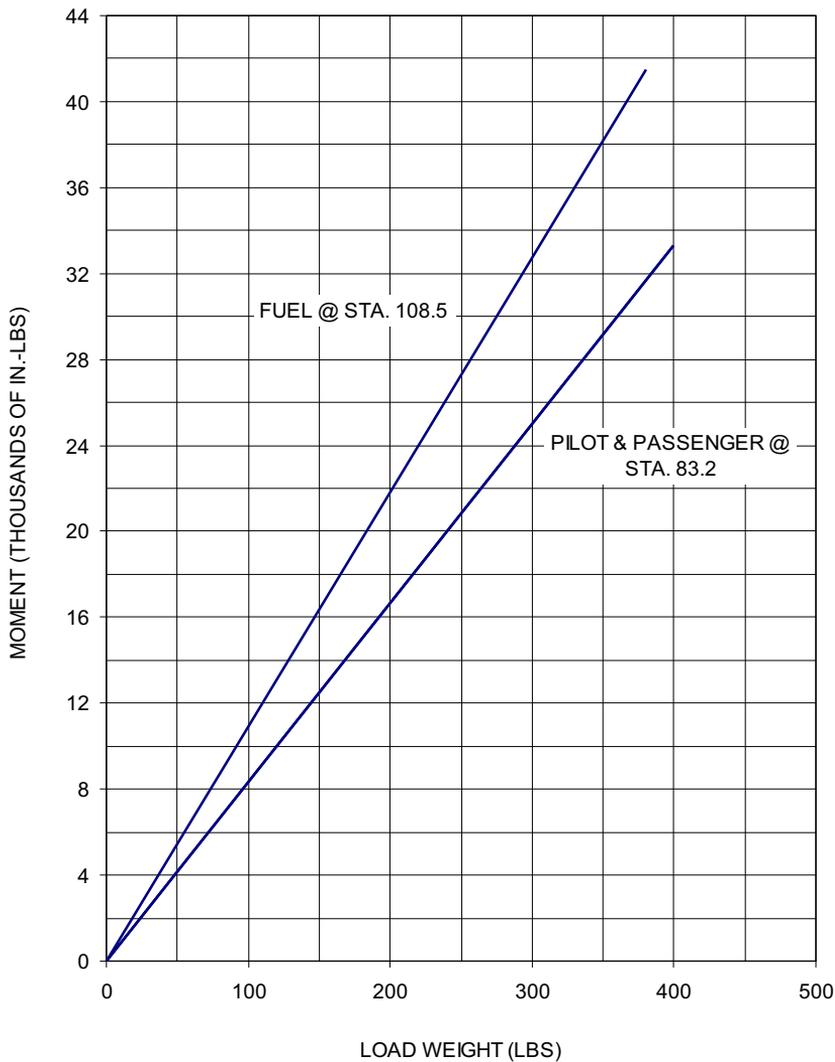
Figure 6-7. Weight and Moment Chart - Longitudinal
