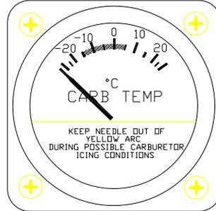
CARB TEMP - Helicopters with carbureted engine (HO-360-C1A)
