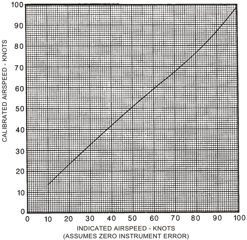
Figure 5-1. Airspeed Calibration Curve - Standard Pitot Tube
