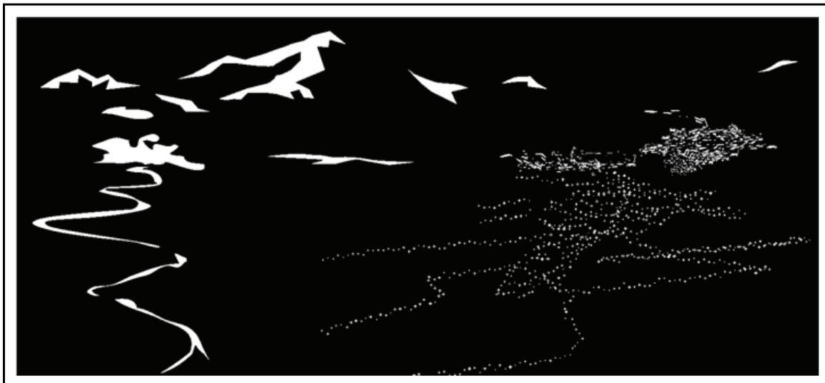
Figure 9-2. Typical light pattern for airport identification
